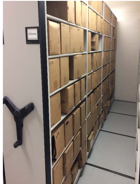
Rolling rack shelving system.
