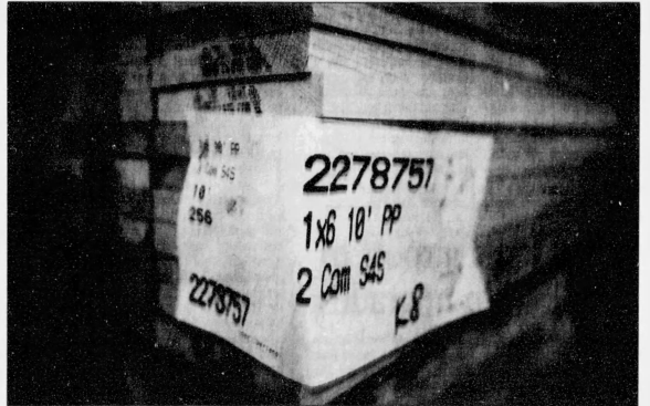
One-by-six-inch boards, measuring 10 feet long, are banded and ready to be shipped to stores for sale
