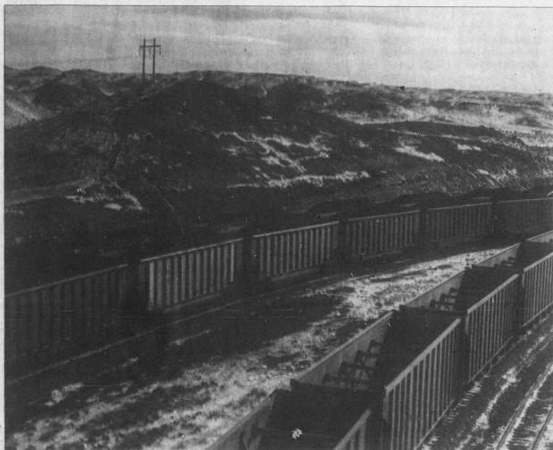
Rail cars are filled with coal and sprayed with a topper agent to suppress dust at Cloud Peak Energy's Antelope Mine north of Douglas. Dependent on environmental review, the proposed Gateway Pacific Terminal project would ship up to 48 million tons of U.S. coal to Asia.
